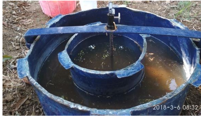
Figure 2. Simple Double Ring Infiltrometer
